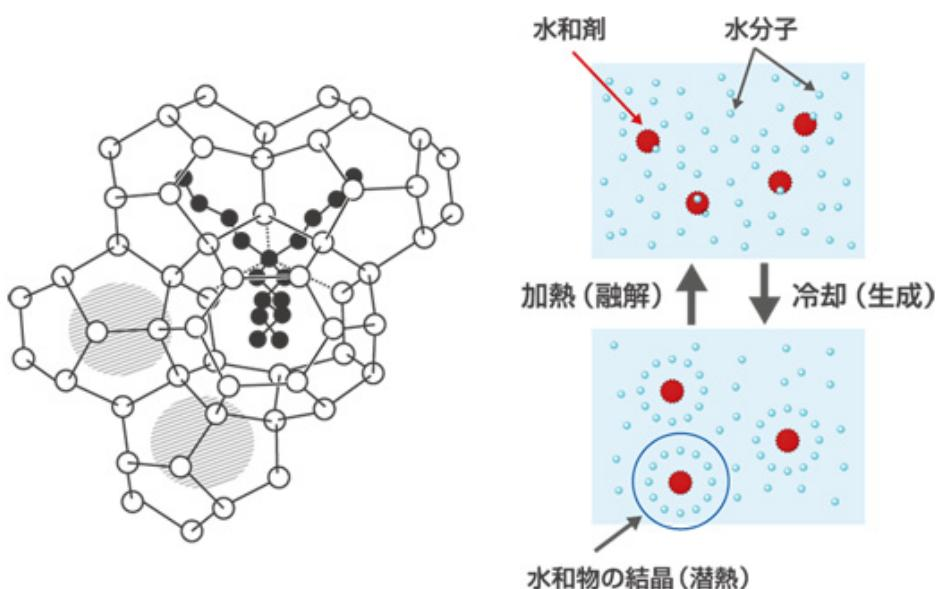
図 TBAB 水和物の構造（左）（W. Shimada, T. Ebinuma, H. Oyama, Y. Kamata, S. Takeya, T. Uchida, J. Nagao and H. Narita, Jpn. J. Appl. Phys., 42 (Pt.2, No.2A), L129, 2003.)
